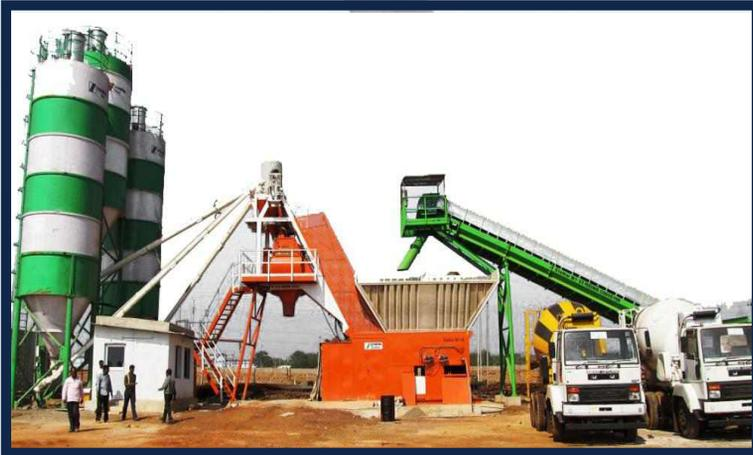
**Concrete Batching Plant**
