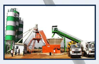
**Concrete Batching Plant**
